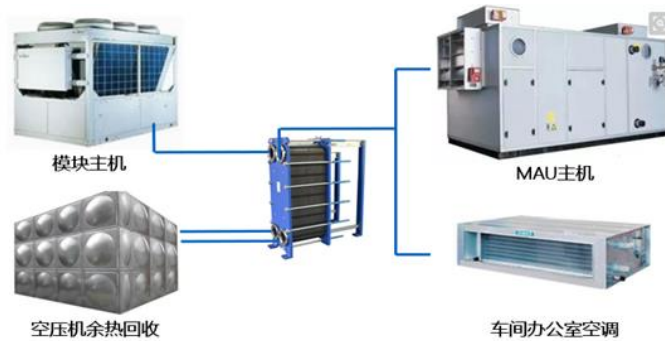
Optimization of 1000 Class Clean Room Air Conditioning (AHU) System
